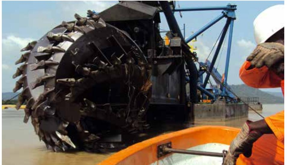
Figure 4. Dredging accuracy remains a challenge to maintain throughout the dredging process – shape and adjustability of suction mouth, cutterhead /suction mouth geometry all have an influence on dredging accuracy.
