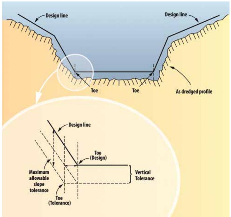
Figure 8. A dredge profile with design level and tolerances.
