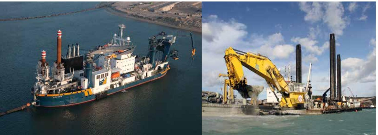
Figure 3. In recent years modern vessels such as the cutter suction dredger (left) and the backhoe (right) have undergone great advancement in horizontal and vertical dredging accuracy.
