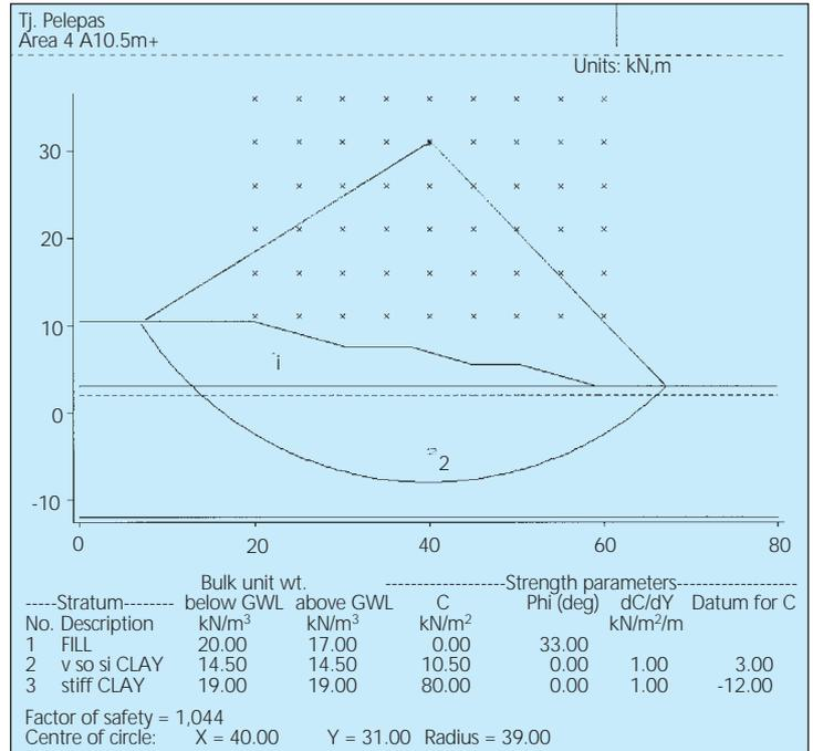
Figure 8. Reclamation slope. Typical slip circle with the minimum safety factor.
